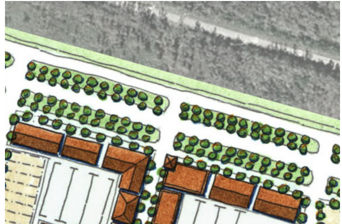
The multi-way boulevard includes multistory, mixed use buildings on wide sidewalks, access lanes for local traffic, medians and travel lanes.
