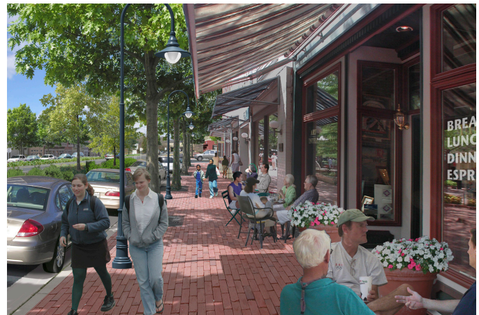
Key locations along multi-way boulevards can feature ample sidewalks for storefronts and patio dining. The pedestrian activity is buffered from the high speed traffic at the center of State Road 82 by an access lane for local traffic and on-street parking.
